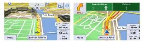
The data fields are different when you are navigating an active route and when you have no specified destination (the orange line is not displayed).
